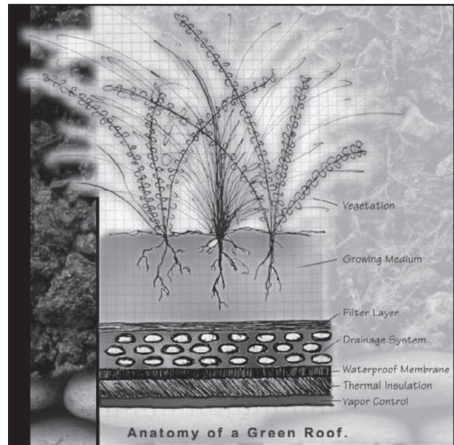
Figure 13. A typical green roof cross section. Image courtesy Green Roofs of Colorado (<http://www.greenroofsco.com/>).
