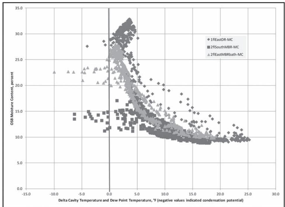
Figure 4. Jobsite 5 comparison of MC and DP. Reprinted with permission, Home Innovation Research Labs; from “High-R Walls for Remodeling: Wall Cavity Moisture Monitoring.” ([http://apps1.eere.energy.gov/buildings/publications/pdfs/building\\_america/high\\_rwalls\\_remodeling.pdf](http://apps1.eere.energy.gov/buildings/publications/pdfs/building_america/high_rwalls_remodeling.pdf))
