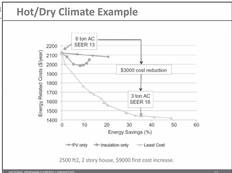
Figure 7. The energy savings in a hot, dry climate that can result from a \$9,000 investment in increased insulation or a \$9,000 investment in a residential PV system, compared with the energy savings that can be achieved by choosing a combination of upgrades that provides the largest overall energy savings. Figure courtesy Ren Anderson, National Renewable Energy Laboratory (NREL).
