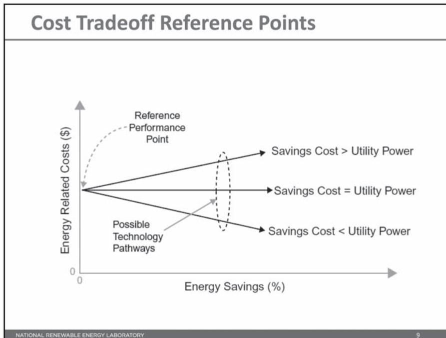
Figure 6. Cost Tradeoff Reference Points. A major question for builders is how best to achieve increases in energy efficiency with the highest reliability, and homeowner value, at the least incremental cost. Figure courtesy Ren Anderson, National Renewable Energy Laboratory (NREL).
