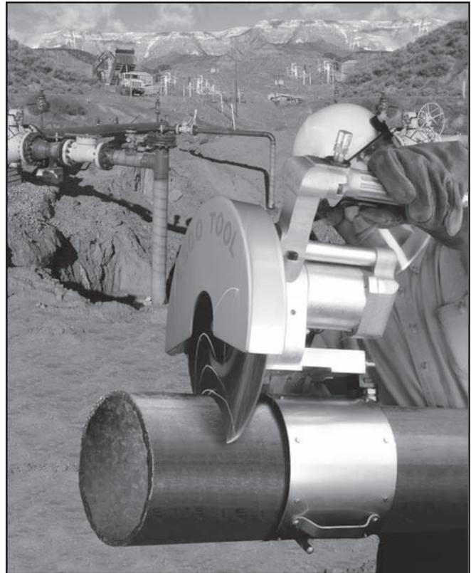
Figure 12. The Esco APS-438 Air Powered Saw and WrapTrack® pipe trolley lets operators rapidly cold cut pipe with  $\pm 1/16$ " accuracy and no HAZ to permit better end prep bevels for welding. Photo courtesy ESCO Tool.
