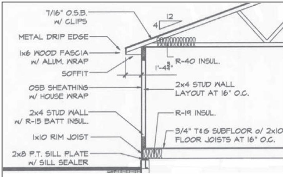
Figure 3. Common wall detail for monitored homes. Reprinted with permission, Home Innovation Research Labs; from “High-R Walls for Remodeling: Wall Cavity Moisture Monitoring.” ([http://apps1.eere.energy.gov/buildings/publications/pdfs/building\\_america/high\\_rwalls\\_remodeling.pdf](http://apps1.eere.energy.gov/buildings/publications/pdfs/building_america/high_rwalls_remodeling.pdf))
